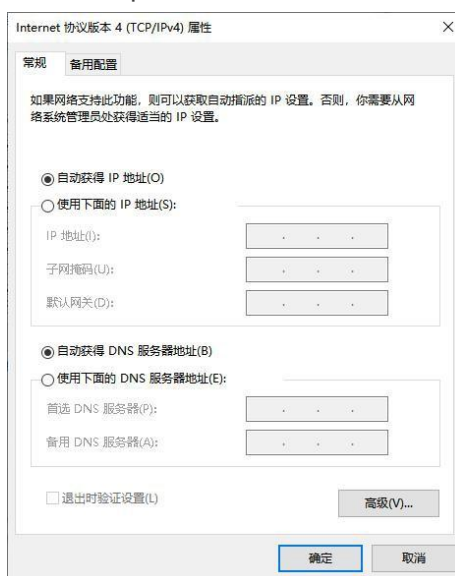
Figure 3-1 PC automatically obtains IP
